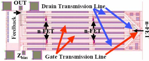
Figure 2. Layout of the monolithic microwave distributed oscillator (top view) in  $0.18\mu\text{m}$  CMOS with G-S-G pads for measurements, chip area:  $1.5 \times 0.65$  sq. mm.
