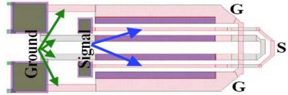
Figure 3. Layout of the coplanar test structure ‘folded CPW’ (top view) used in the bend path of the gate line.
