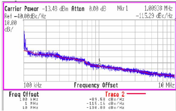
Fig. 6. Measured phase noise spectrum of the Osc-1. It is -115.16dBc/Hz at 1 MHz offset from the carrier.
