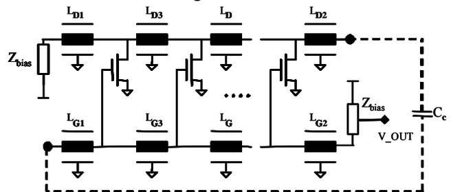
Figure 1. Schematic of the DO with coupling capacitor  $C_c$  incorporated in simulation after measurements.
