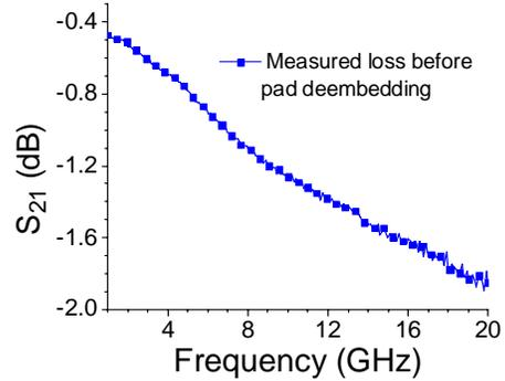
Figure 4. Measured loss  $S_{21}$  (dB) versus frequency of the coplanar test structure of Figure 3.
