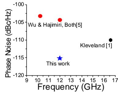
Figure 7. Comparison of measured phase noises for DOs. dBm increase in output level. By decreasing the gate voltage by 0.2V while keeping the drain voltage constant at 1.8V, the frequency is increased by 60MHz with a 1.3dBm decrease in output. We observe that this design variation results in a high frequency VCO with large amplitude, achieved by tuning the parasitic gate and drain capacitances (“inherent varactors” [5]) of the n-FETs.
