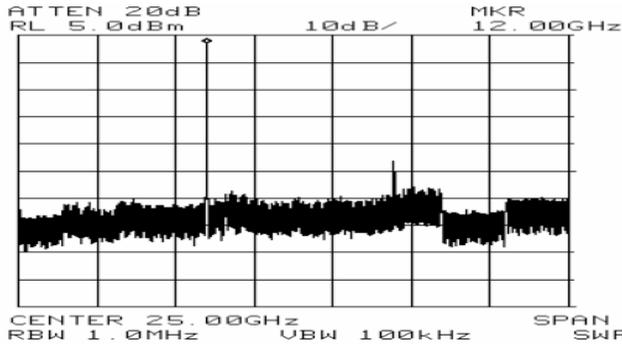
Figure 5. Measured power spectrum of the Osc-1 with marker showing that the fundamental is at 12.00GHz, +5.77dBm (includes 2.6dB loss from the testing systems). implemented in industry-standard silicon CMOS are compared to prior reported results (implemented with non-standard CMOS [1] and BiCMOS [5] processes) in Table 1 and Figure 7 respectively. OSC-1 offers the best power and phase noise results of DOs in the literature.
