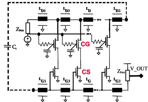
Figure 8. DO with n-FET cascode gain cells. source stage with a common gate stage, as in [4], [6]. The
