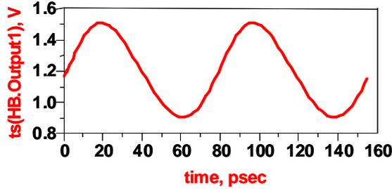
Figure 9. Time domain waveform of OSC-2.
