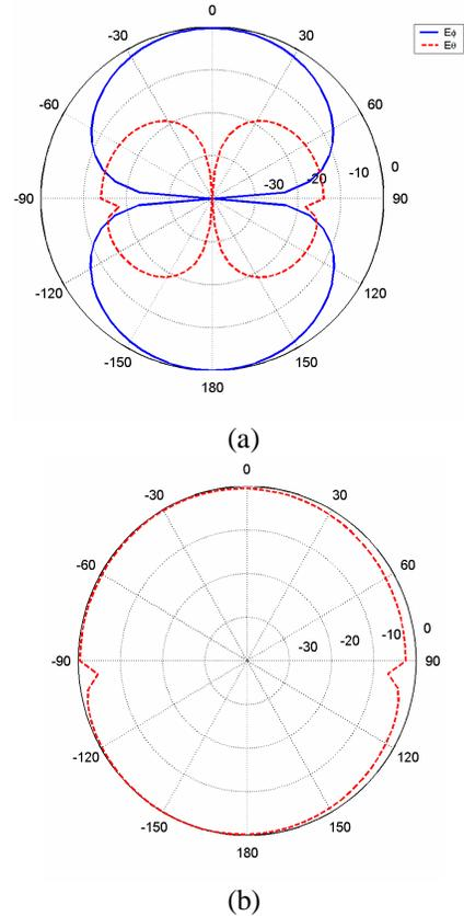
**Figure 6: Computed normalized radiation patterns ( $R = 10$  mm,  $h = 1.5$  mm,  $t = 13$  mm) at 5 GHz, (a)  $\phi = 0^\circ$  and (b)  $\phi = 90^\circ$ .**
