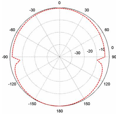
**Figure 8: Computed normalized radiation patterns ( $R = 10$  mm,  $h = 1.5$  mm,  $t = 13$  mm) at 7 GHz,  $\phi = 90^\circ$ .**
