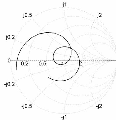
**Figure 4: Input impedance of the slot antenna ( $R = 10$  mm,  $h = 1.5$  mm,  $t = 13$  mm).**
