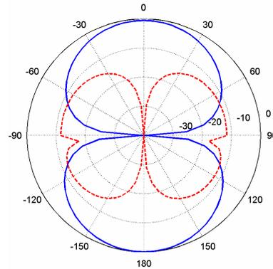
**Figure 7: Computed normalized radiation patterns ( $R = 10$  mm,  $h = 1.5$  mm,  $t = 13$  mm) at 7 GHz,  $\phi = 0^\circ$ .**
