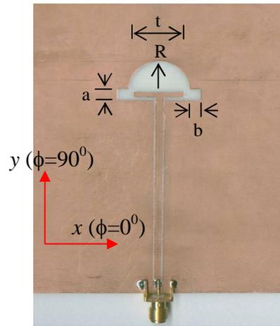
**Figure 1: Photograph of CPW-fed wide-band slot antenna ( $R = 10$  mm,  $h = 1.5$  mm,  $t = 13$  mm,  $a = 5$  mm, and  $b = 2.5$  mm).**
