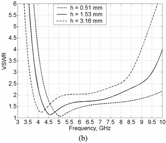
**Figure 2: Computed VSWR with (a) circle radius and (b) substrate thickness as parameters.**
