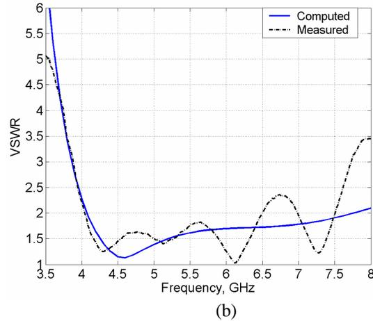
**Figure 3: (a) Computed VSWR with varying tuning stub length and (b) computed and measured VSWR characteristics ( $R = 10$  mm,  $h = 1.5$  mm).**
