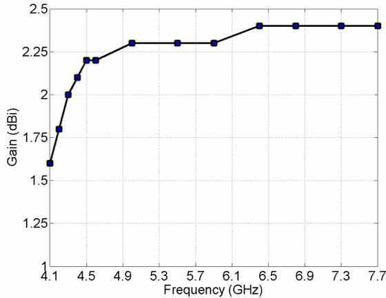
**Figure 5: Computed gain as a function of the operating frequency ( $R = 10$  mm,  $h = 1.5$  mm,  $t = 13$  mm).**
